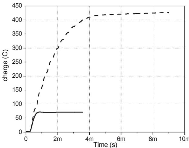
**Figure 3.** Charges through the switch (solid line: nominal operation, dash line: short-circuit case at 16 kV charging voltage).
