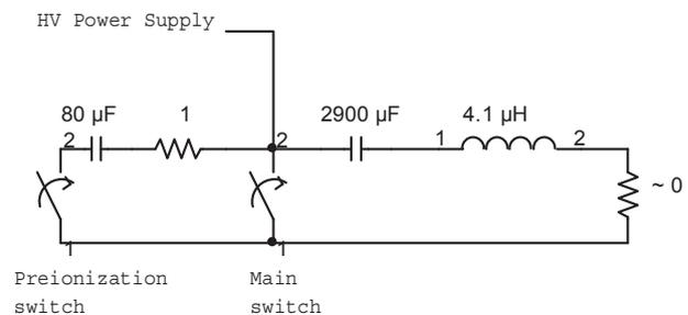
Figure 1. Equivalent circuit for the short-circuit tests
