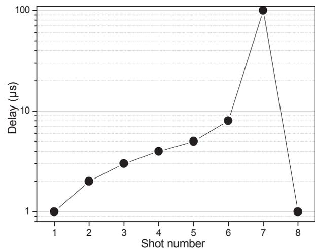
**Figure 4.** Evolution of the delay between the trigger and the rise of the current on the main switch. The switch wasn't purged after shot 1 to 6. The purge was restarted after the seventh shot.
