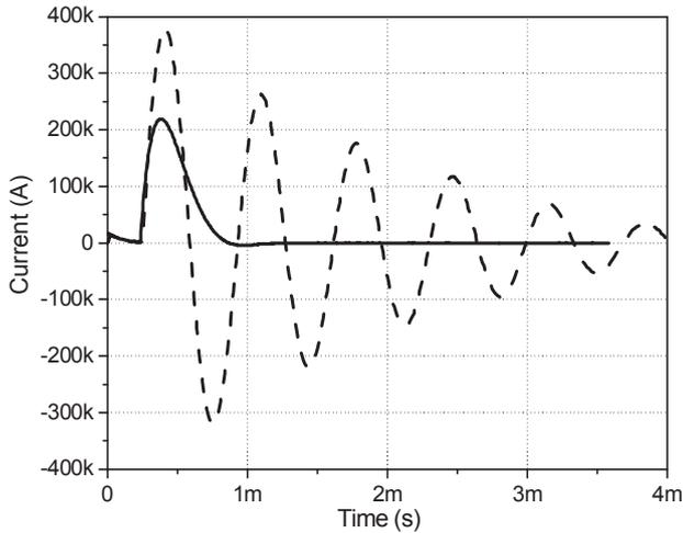
**Figure 2.** Current through the switch (solid line: nominal current at 24 kV, dash line: short-circuit current for 16 kV charging voltage).
