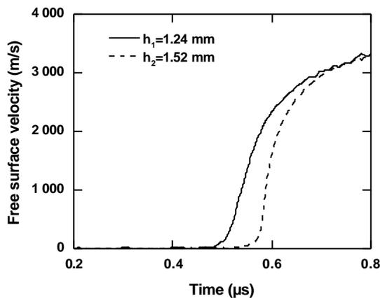
FIGURE 4. Free surface velocity diagrams obtained on two copper samples (shot #252). The width  $W$  of the line is 5 mm.
