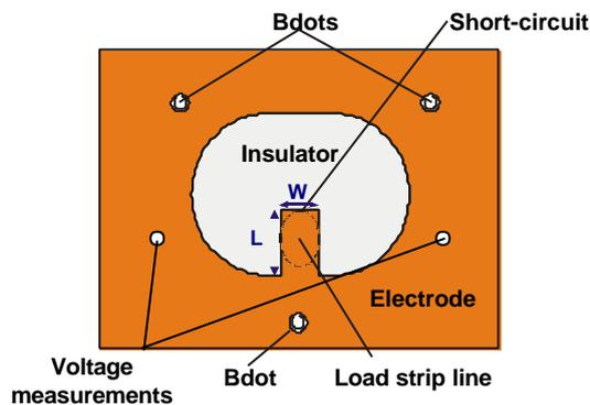
FIGURE 2. Scheme of an electrode in the load region .
