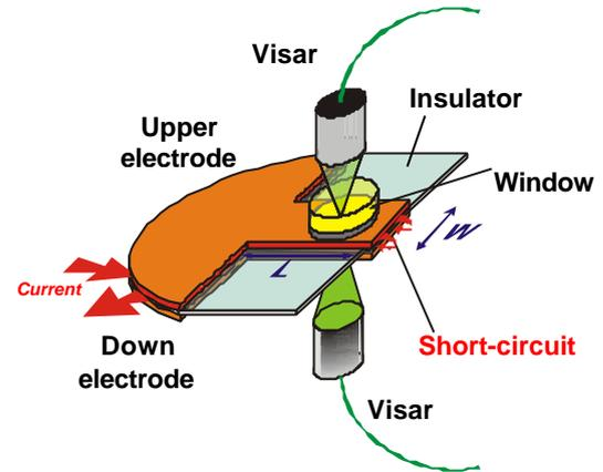
FIGURE 3. VISAR measurements on samples.
