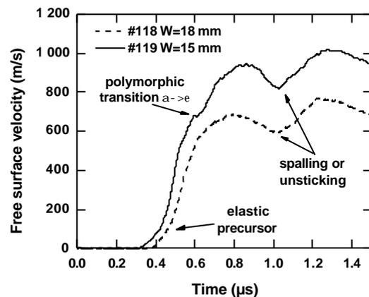
FIGURE 6. Free surface velocities diagrams obtained on iron sample showing the  $\alpha$ - $\epsilon$  transition at 13 GPa.
