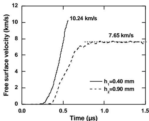
**FIGURE 7.** High velocity aluminum flyer plates obtained with a line width of 6 mm. Sample thicknesses are 0.40 mm and 0.90 mm.
