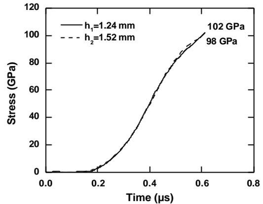
FIGURE 5. Stress diagrams on copper calculated with backward method for shot #252.
