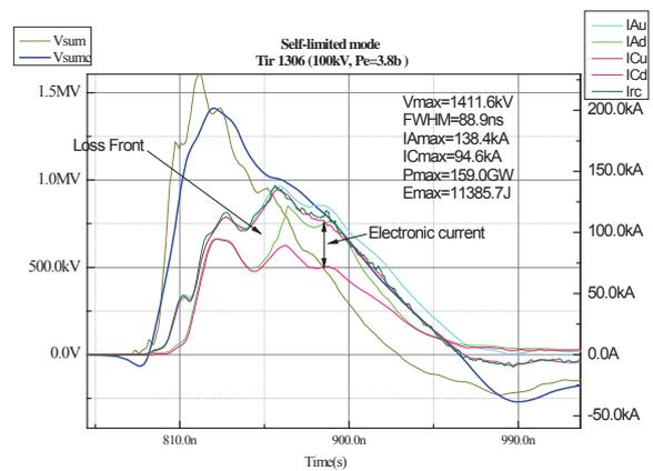
**Figure 9.** Graph of the typical output data on the 1MV generator in self limited MITL mode (~8Ω)
