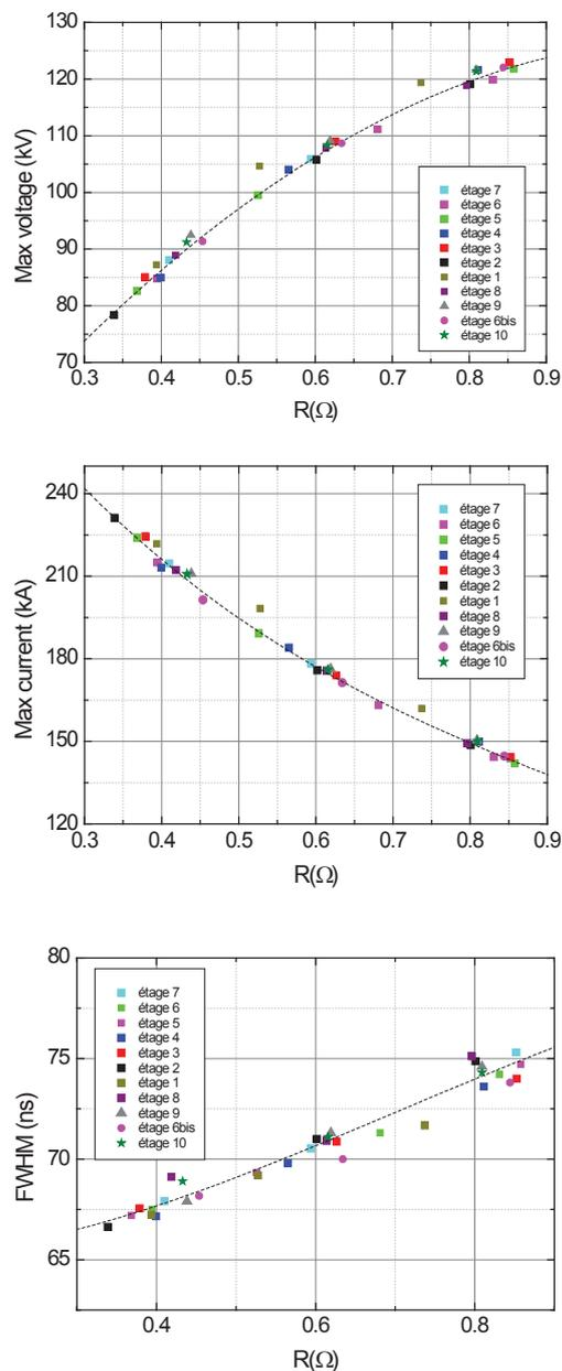
Figure 2. Synthesis of the output parameters (V, I, FWHM) of the 10 stages.
