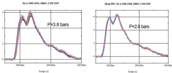
**Figure 11.** Comparison of 20 consecutive X-ray pulses at 3.8bars and 2.8 bars pressure in the switches.
