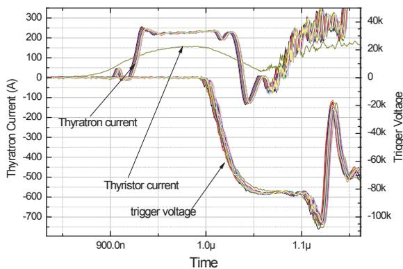
**Figure 6.** Graph showing the overall jitter of the thyatron discharge currents and trigger output voltages over 20 shots.
