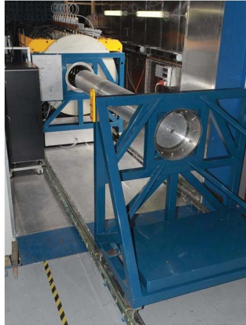
**Figure 4.** View of the cathode and its support moving on rails outside from the generator.
