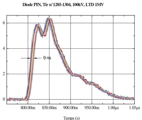
**Figure 10.** Superposition of the X-ray pulses on 20 consecutive shots at 3.8bars pressure in the switches
