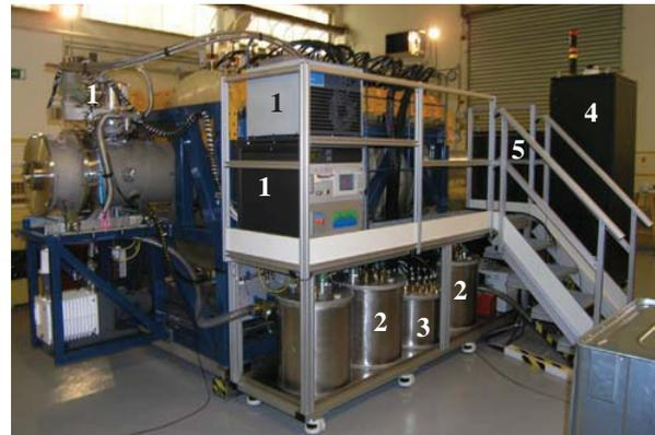
**Figure 5.** View of the subsets of the 1MV generator (1 - vacuum systems, 2 - HV distribution and dump, 3 - HV trigger, 4 - command-control, and 5 - acquisition bay) integrated on a lateral support.
