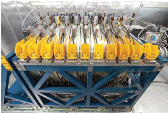
**Figure 3.** Overall view of the 1MV generator made by 10 LTD cavities stacked in series on a metal stand
