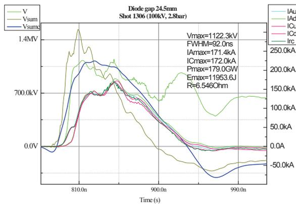
**Figure 8.** Graph of the typical output data of the 1MV generator on a 6 Ω large area diode (IAu,d and ICu,d anode and cathode current, upstream: after stage 10 and, downstream: just before the diode).
