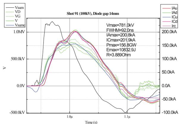
**Figure 7.** Graph of the comparison of the measured voltage (in green, VD, VG) by 2 capacitive monitors, and mean value (V) compared to the calculated one (Vsumc in blue) from the sum of the stages voltage (Vsum in black) and generator currents (right axis).
